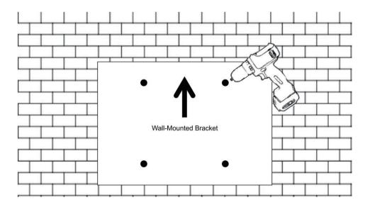
**Use 4 sets** Hexagonal Expansion Screws to secure the wall-mounted bracket on the wall.
